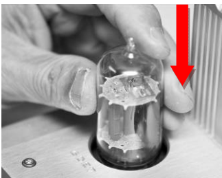
Insert the tube perpendicular to the socket
