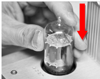
Insert the tube perpendicularly to the tube socket
