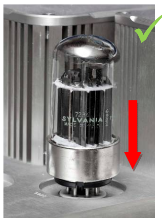
Insert a tube perpendicular to the socket.
