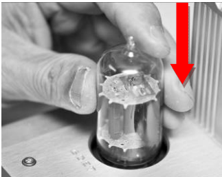
Insert the tube perpendicular to the socket
