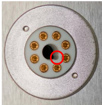
Tube socket guide pin indicator
