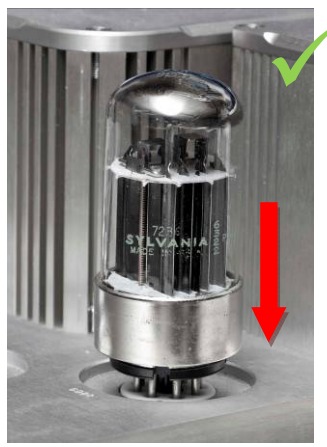
Insert a tube perpendicular to the socket.
