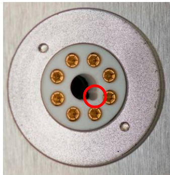
Tube socket guide pin indicator
