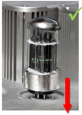
Insert a tube perpendicular to the socket.
