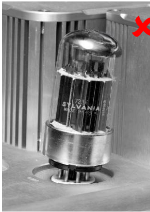
Do not insert a tube at an angle
