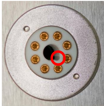
Tube socket guide pin indicator
