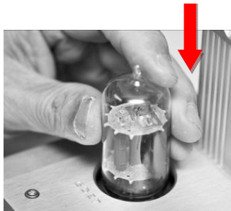
Insert the tube perpendicular to the socket
