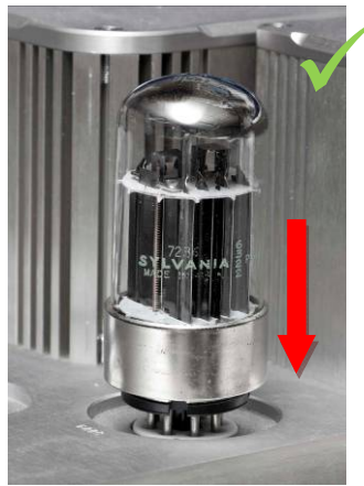
Insert a tube perpendicular to the socket.
