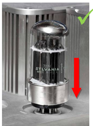
Insert a tube perpendicular to the socket.
