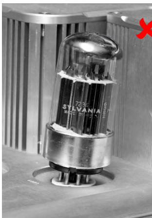
Do no insert a tube at an angle
