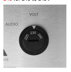
To change the voltage switch, be sure the unit is switched off, insert a Philips flat screwdriver to the slot then turn to the number to the arrow.
