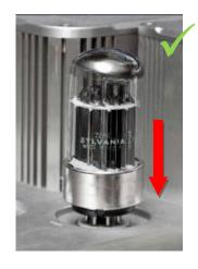
Insert a tube perpendicular to the socket.
