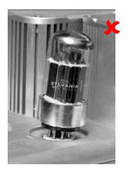
Do no insert a tube at an angle
