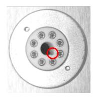
Tube socket guide pin indicator
